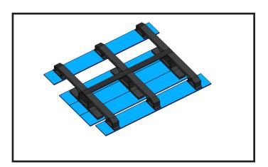
5. With the aide of another person, flip the table 180° so that the table top is resting on the ground. Place the center support in the grooved notch and fasten the support using the 3-1/2" lag screws and washers.
