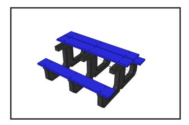
4. Loosely attach table slats to plastic base with the 4" lag screws using the socket wrench. Make sure to lay them all on top first to line them up. Then pre drill starter holes.
