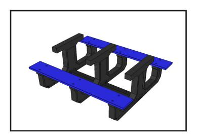
3. Place one seat slat on each side of the base. With the bases in the vertical position, pre-drill two holes on both ends of each seat slat with a 3/8" drill bit.
