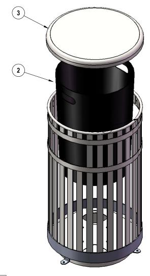
Recommended Surface Mount Hardware: 3/8" x 3-1/2" Concrete Expansion Anchor Bolts (Not Included)
