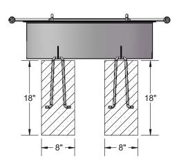
Attach the ground staples to the Fire Ring before inserting then into the concrete footings.
