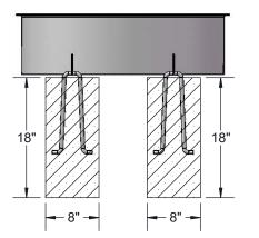
Attach the ground staples to the Fire Ring before inserting then into the concrete footings.
