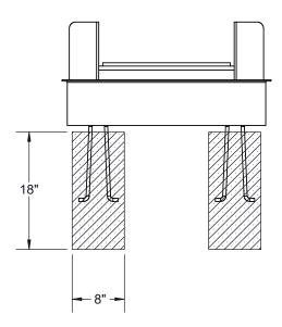
Attach the ground staples to the Fire Ring before inserting then into the concrete footings.
