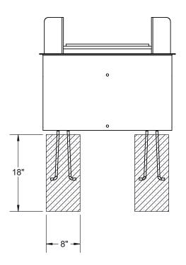
Attach the ground staples to the Fire Ring before inserting then into the concrete footings.
