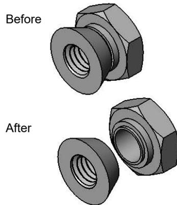
Hex part of nut will break off when tightened to 185in-lbs.
