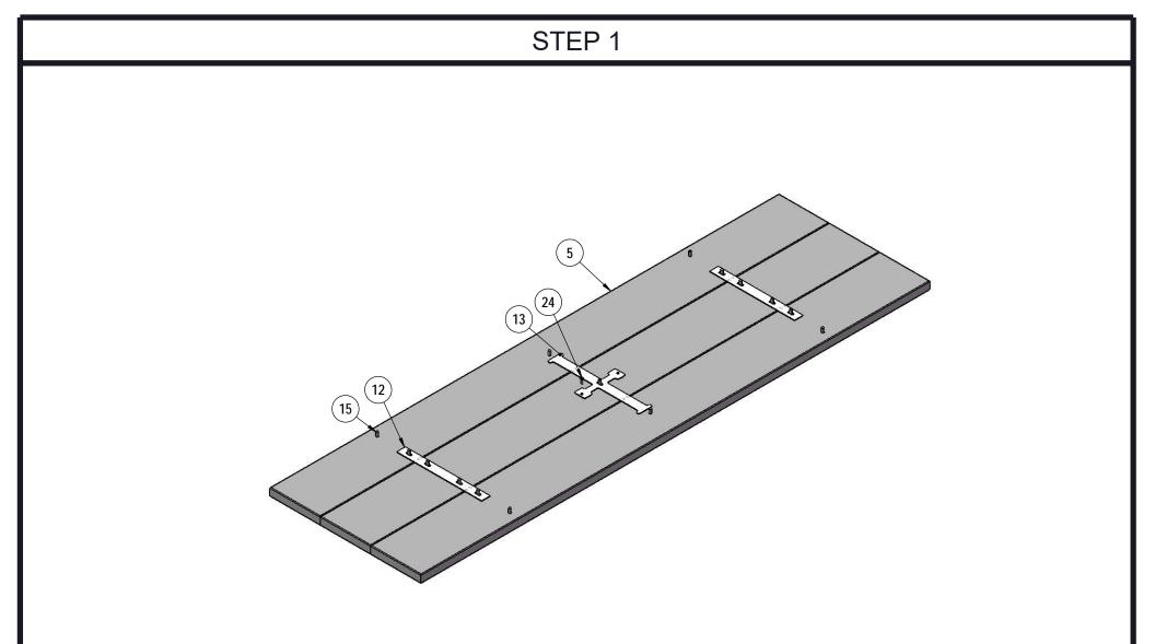
Insert the 5/16" x 2-1/4" Carriage Bolts through 3 Recycled Planks for the top. Place the Table Top Center Strips and Center Cross Spacer Plate on the corresponding hardware like shown. Attach the Center Cross Spacer Plate with a #14 x 1" Wood Screw.
