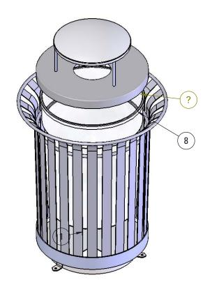
Optional Surface Mount Hardware: 3/8" x 3-1/2" Concrete Expansion Anchor Bolts (Not Included)
