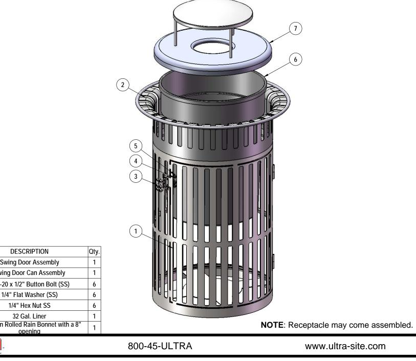
ITEM NO. PartNo Swing Door Assembly 01-05-0221 1 01-05-0220 Swing Door Can Assembly 2 33-06-0075 1/4"-20 x 1/2" Button Bolt (SS) 3 33-02-0016 1/4" Flat Washer (SS) 4 5 33-01-0036 PL-32 6 32 Gallon Rolled Rain Bonnet with a 8" RBR-32-08 7 ultra site
